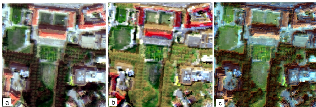
Figure 17 Pan-sharpened hyperspectral images using (a) Gram-Schmidt, (b) PC, and (c) Wavelet-PC. PC: principal component.
