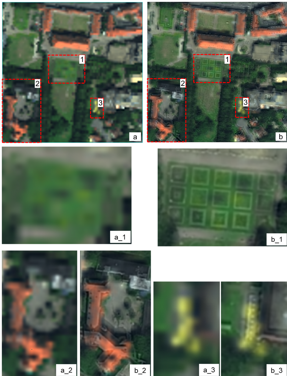
Figure 18 Using simplified Ehlers fusion to sharpen hyperspectral image: (a) original hyperspectral image with the true color display where RGB bands are represented by band 15, band 9, and band 4 respectively; (b) fused image with the same color display; (a_1, b_1, a_2, b_2, a_3, b_3) magnified areas marked in (a) and (b). RGB: red, green, and blue.
