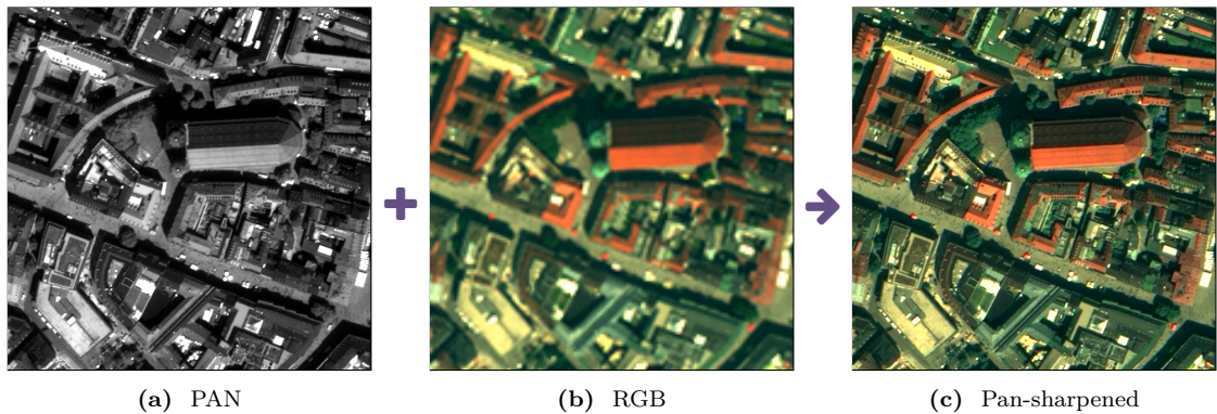
Figure 2.3: An example of (a) PAN image with Ground Sampling Distance (GSD) of 0.5 m, (b) red, green, and blue (RGB) image with GSD of 2 m, and (c) pan-sharpened image with GSD of 0.5 m depicting a central cathedral in the city of Munich, Germany. Images are acquired with WorldView-2 satellite. The pan-sharpened image is generated by combining the high-resolution pan-chromatic image with low-resolution RGB image using a pan-sharpening technique developed by Krauß et al. [7].
