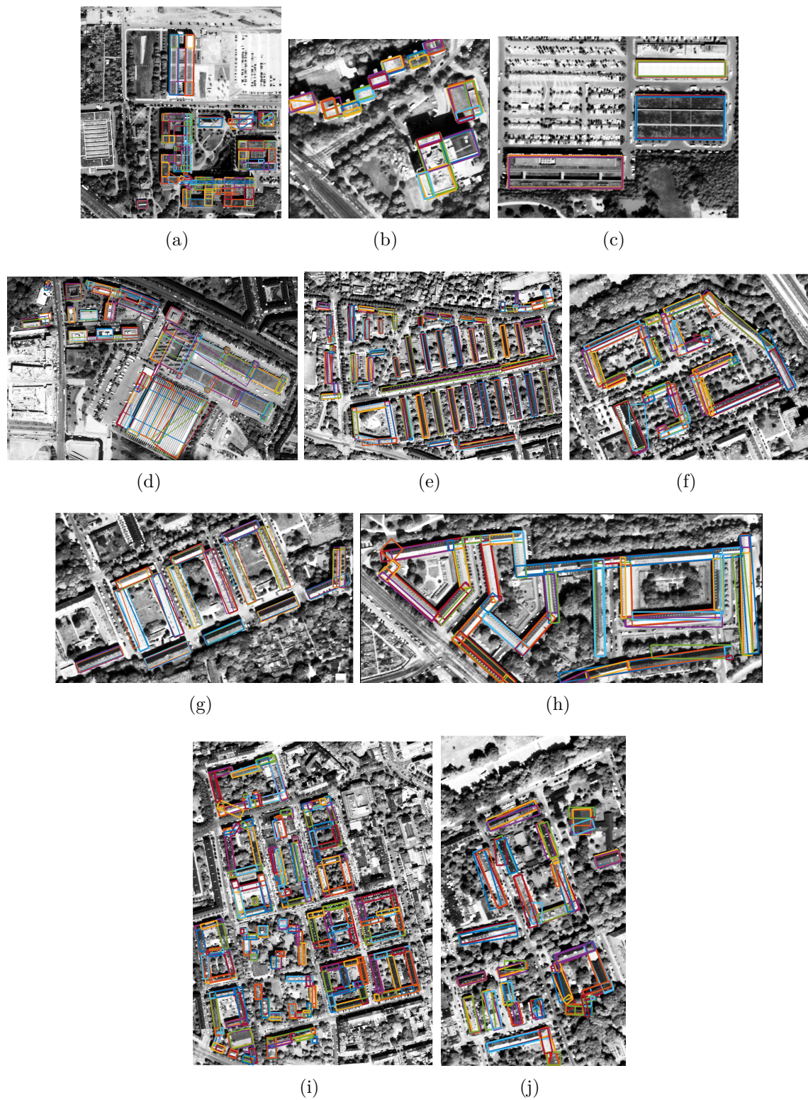
Figure 3.15: Illustration of decomposed building outlines into rectangular shapes, (a) I_1 , (b) I_3 , (c) I_2 , (d) I_{10} , (e) I_8 , (f) I_6 , (g) I_7 , (h) I_4 , (i) I_9 , (j) I_5
