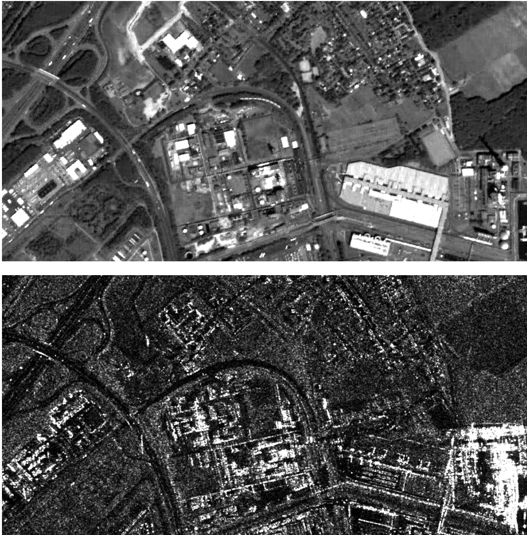
Figure 1.1: Illustration of an optical (top) and SAR image (bottom) covering the same area. Both images have a ground sampling distance of 1.25 m.
