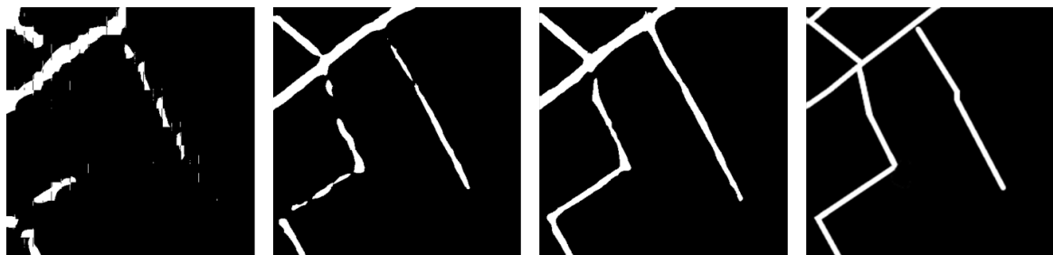
Figure 4.6: Segmentation result comparison between three the FCN versions (left to right: FCN32s, FCN16s, FCN8s, ground truth)
