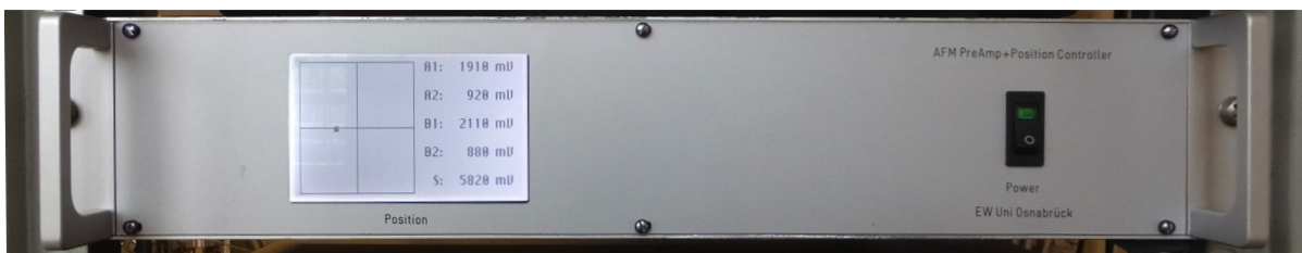
Fig. 3.7: Photo of the new home build pre-amplifier with display for the positioning of the laser spot on the photodiode.
