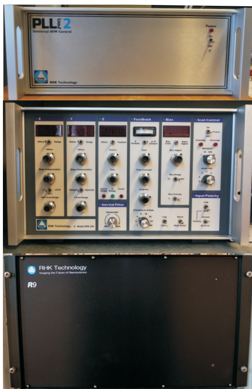
Fig. 3.12: The photograph shows the two RHK scan controller systems, namely the SPM 1000 with the PllPro2 and the R9. The most obvious difference between the two systems is that the R9 does not have analog potentiometers for adjusting scan parameters. One example is the z-feedback which in the SPM 1000 consist of two potentiometer (gain and time constant) and is now integrated in the software, allowing a more precise adjustment.
