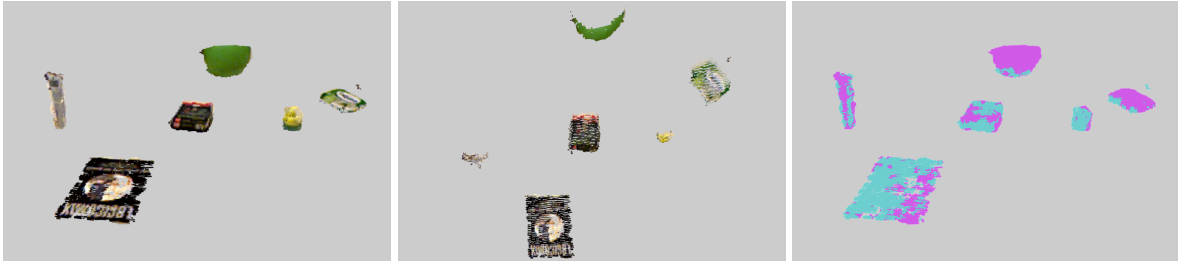
Figure 5.37: Violation of data assumption, overview: display of the complete scene, first in perspective and top down view with color information. Points in the image on the right are colored according to the original point cloud. All three images suggest good alignment, similar to Figure 5.34.
