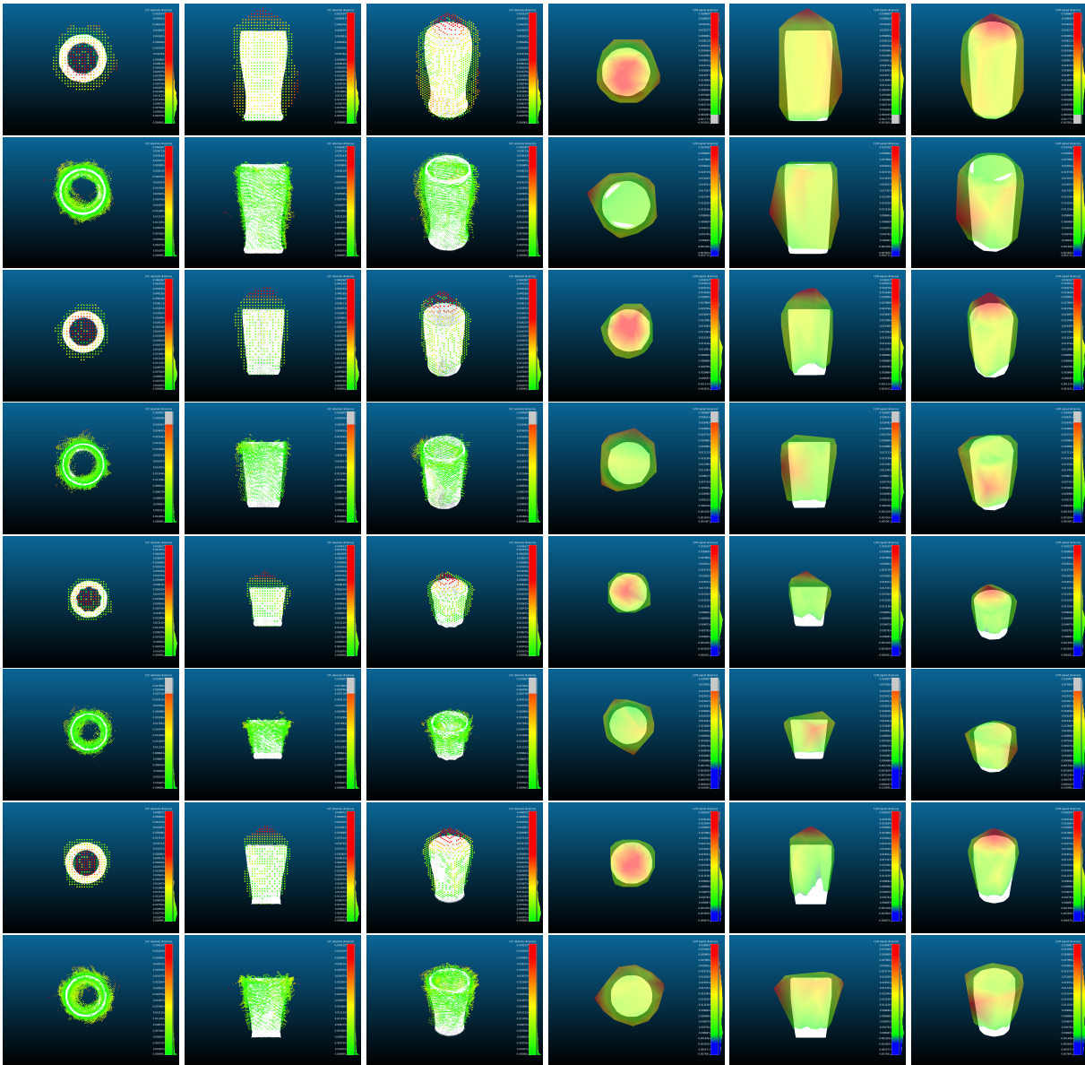
Figure A.2: Comparison viewpoint-based reconstruction glass1 , glass3 – glass5 . Each row from left to right: Top view point cloud comparison; side view, point cloud; perspective view, point cloud; top view convex hull mesh; side view convex hull; perspective view convex hull. From top to bottom: Rows come in pairs, with the first row displaying the results of the viewpoint-based reconstruction and the second the reconstruction result from the painted counterpart in the scene. From top to bottom: glass1 , glass3 , glass4 and glass5 .
