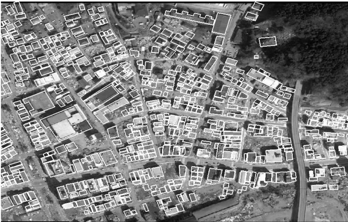
Figure 5.1: The first study case: post-event image of Kamaishi, Japan overlaid with vector data containing building footprints. The satellite image is courtesy of Digital Globe (©Digital Globe 2013); vector data are provided by OpenStreetMap (© OpenStreetMap contributors).
