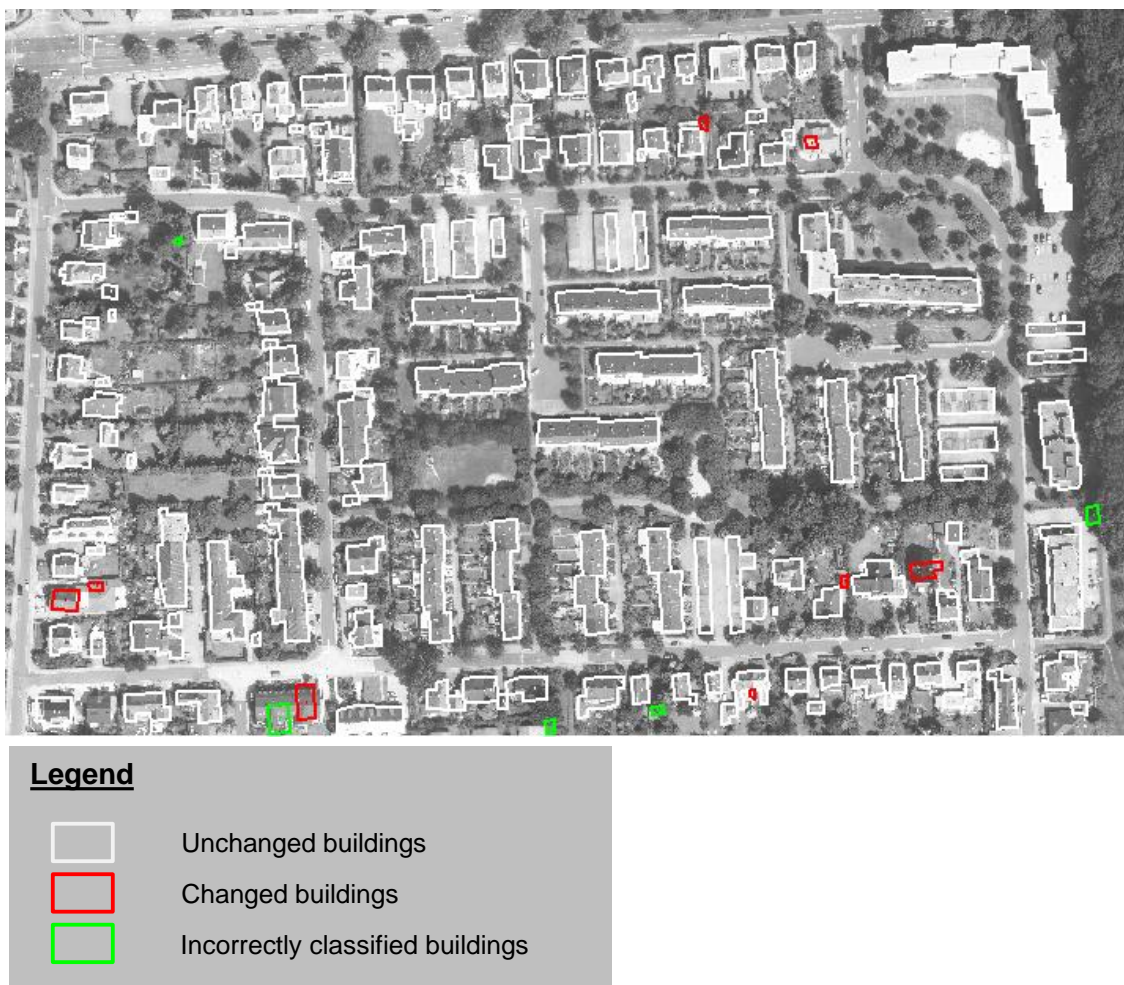
Figure 5.25: Resulting damage map generated for the study case Osnabrueck (Germany): white objects represent intact buildings, red – destroyed; and green objects correspond to the incorrectly classified buildings.
