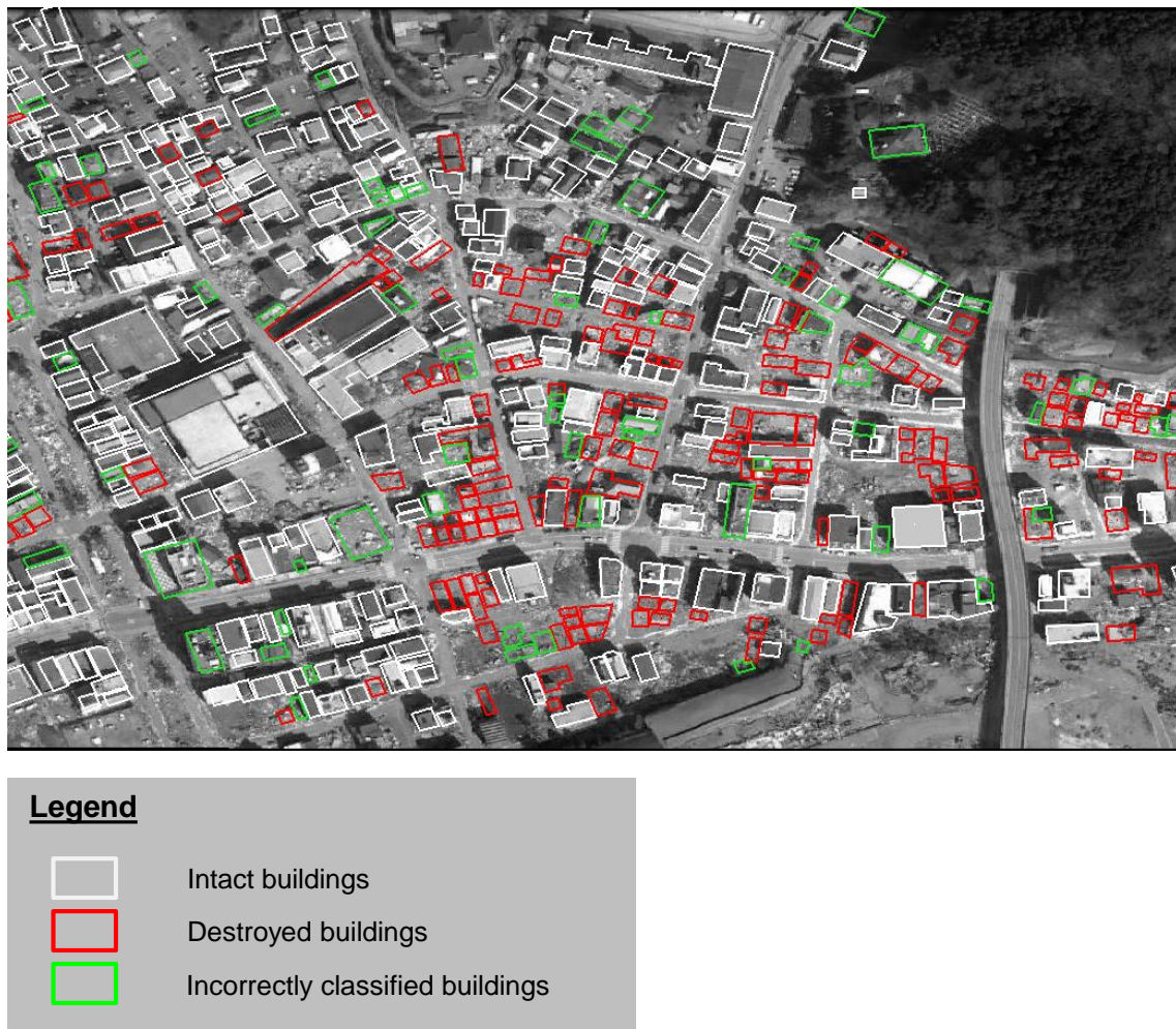
Figure 5.12: Resulting damage map generated from the results obtained by SVM classification for the study case Kamaishi, Japan (the 2011 Tohoku earthquake): white objects represent intact buildings, red – destroyed, and green objects correspond to the incorrectly classified objects.
