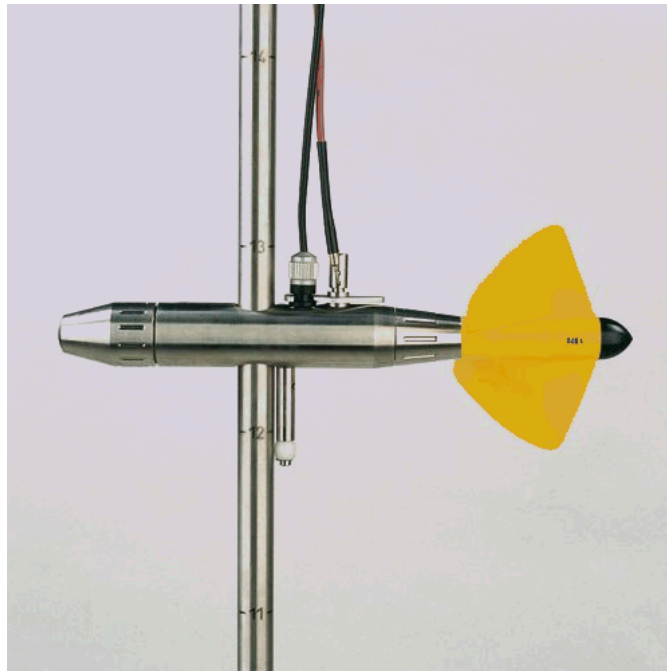
Figure 7. Current meter with propeller, range 0.025-10 m/s (adopted from http://pkd.eijkelkamp.com ).
