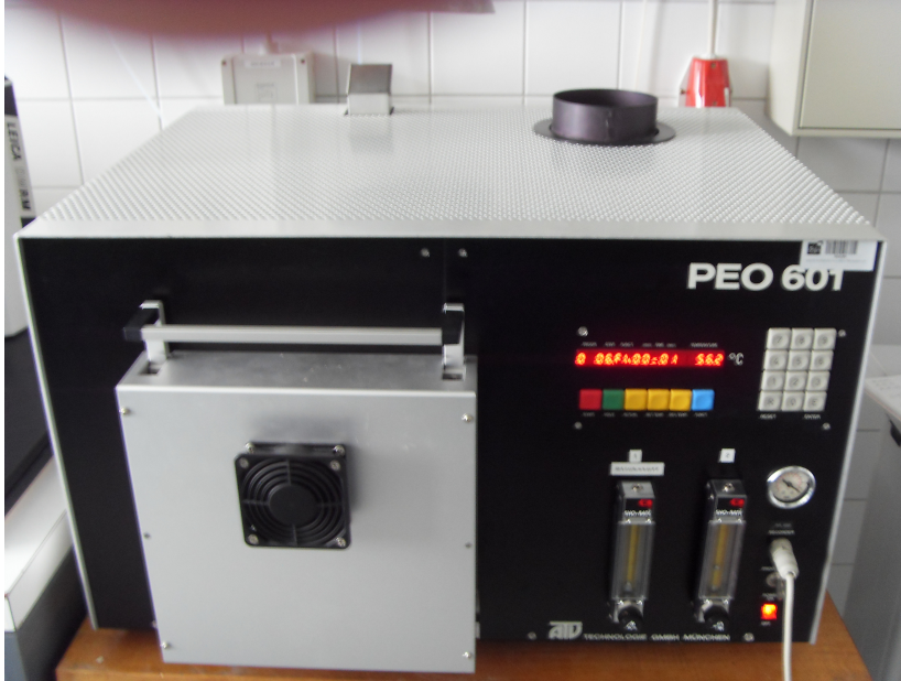
Figure 3.2: Furnace for post deposition annealing of the samples in oxygen. Temperatures were varied from sample to sample and the annealing time was 30 minutes.
