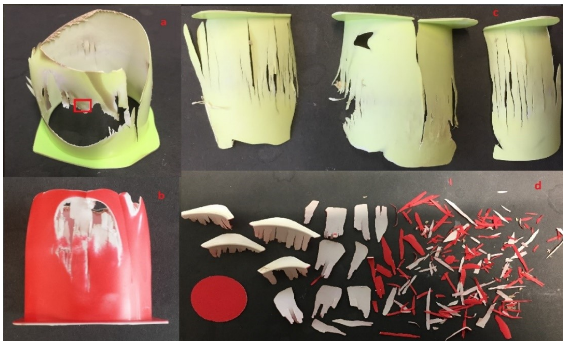
Figure 32: Effects of mechanical stress detected by PS cup samples exposed in BE.
