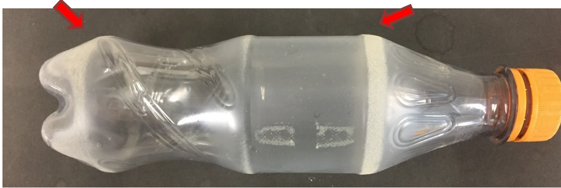
Figure 26: Effects of mechanical stress detected by PET bottle samples exposed in WTE.
