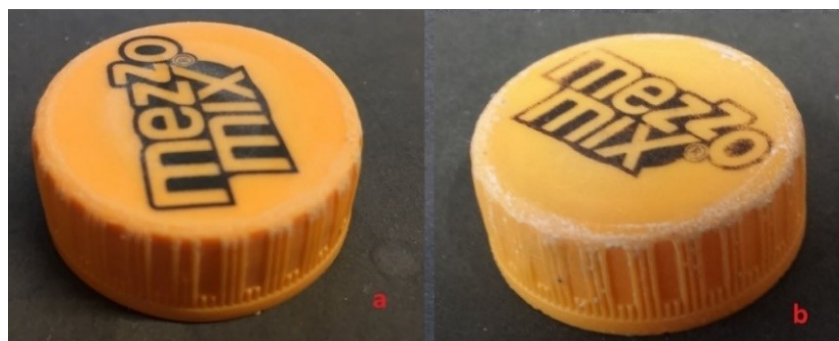
Figure 29: Effects of mechanical stress detected by PE cap samples exposed in WTE.
