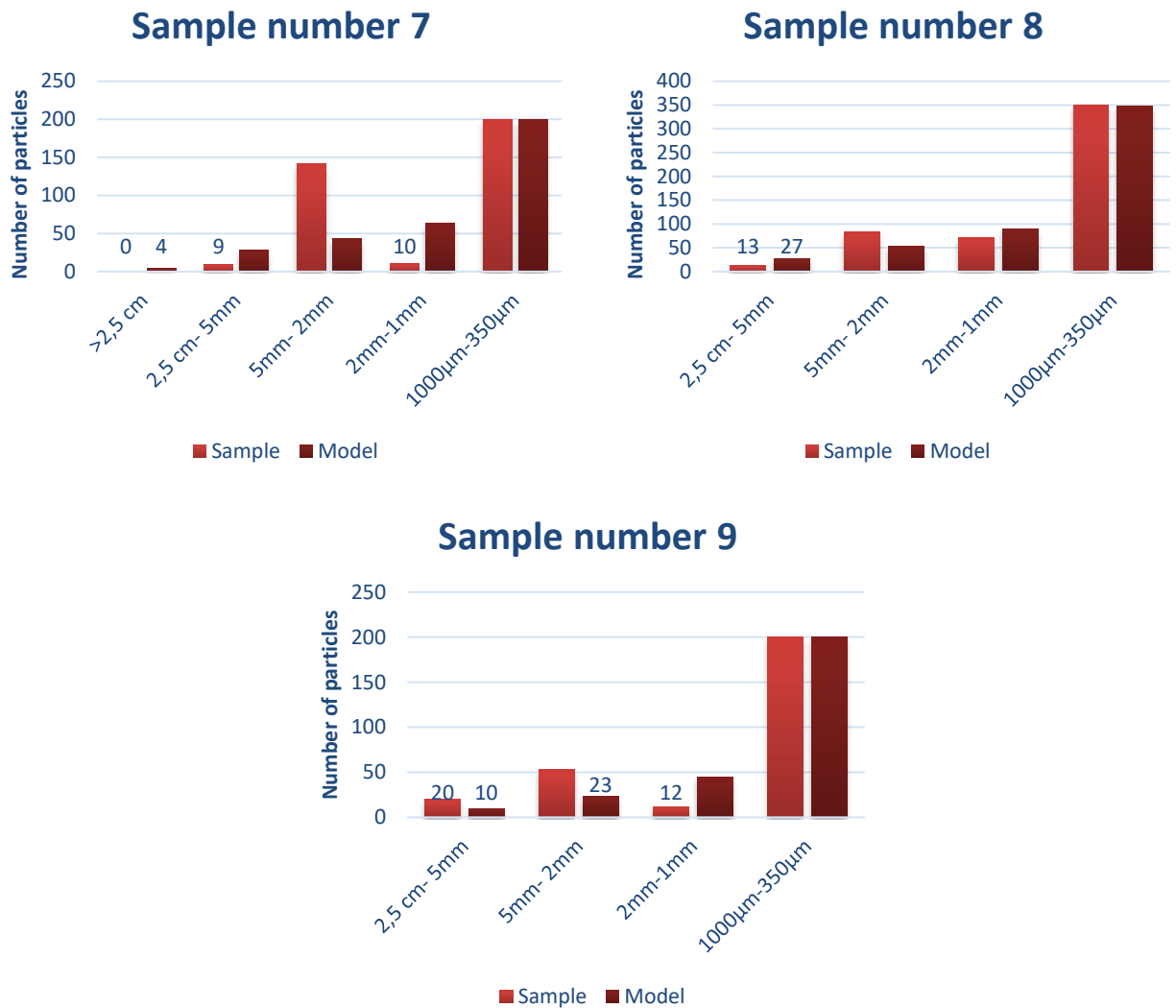
Figure 46: Counted particle size distribution of samples 1-9 in five four size classes, respectively, compared to distributions modelled with the power law model.
