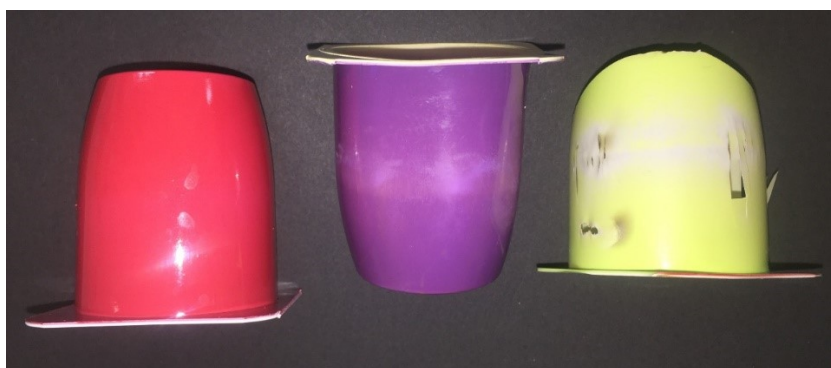
Figure 23: Example of PS cup samples in the three different abrasion categories. Red sample: Abrasion category 0; Purple sample: Abrasion category 1; Yellow sample: Abrasion category 2.
