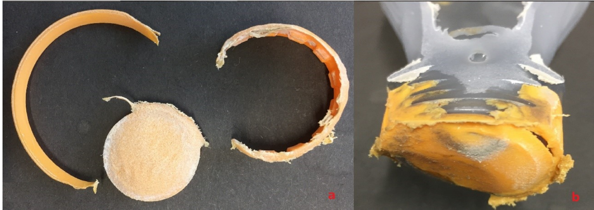
Figure 28: Effects of mechanical stress detected by PE cap samples exposed in BE.
