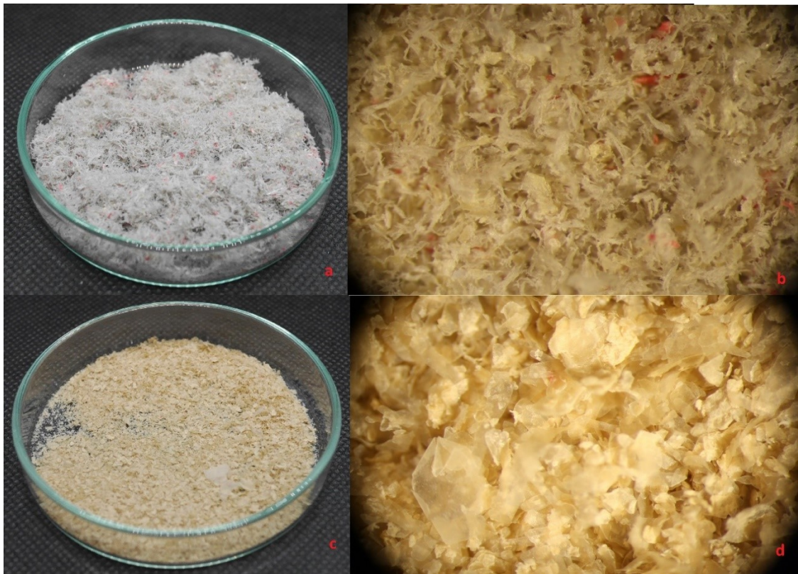
Figure 36: Fragmentation pattern of LDPE bag samples. In a and b (magnification of x25) sample cakes from LDPE bags with damage pattern 2b are shown. C and d (magnification of x25) show sample cakes from samples with damage pattern 2c.
