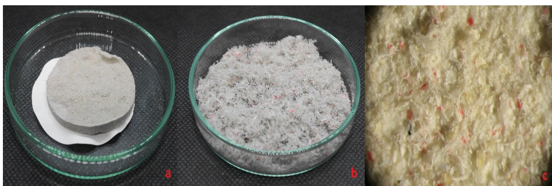
Figure 18: PE bag sample cake forming an entanglement after extraction (a). Entanglement was carefully released (b). Sample section with a x40 magnification (c). Red particles were PS sample microplastics trapped in the LDPE-entanglement.
